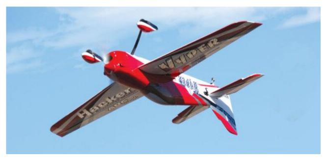
Flying an aircraft upside-down can be challenging. Typically, this is because you need to push on the elevator stick and apply down-elevator to maintain altitude, which may seem odd at first. Depending on the bank angle that is established at the start of the maneuver, rudder input is needed to maintain altitude as higher bank angles require larger amounts of rudder. Like all things in life, though, these control inputs will become second nature with proper practice techniques.
